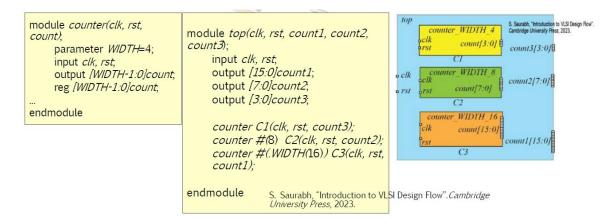
Now, during instantiation, we can change the value of the parameters. For example, in this instance, C1, we are not changing. So in this case the default value of 4 will be used for count3 for the instance C1. For the another instance, C2, we are saying that instead of 4, use a value of WIDTH as 8. So in this case, the width of the bus, width of the port count will be 8 instead of 4.
