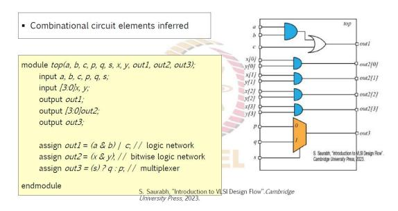
So first, let us look into the assign statement. So how is a continuous assignment or assign statement synthesized if it exists in the RTL code. So, corresponding to the assign statement, a combinational circuit will be inferred, and what combinational circuit will be inferred will depend on what is on the RHS of the assigned statement. So, let us take an example and understand this. Suppose there is a module top and in which we have say three assign statements.
