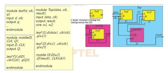
So this is an instance, instantiation of leaf. So we say that for this instance F1, F1 is the name of the instance, the master module is leaf because the name here is referring to this other module. So the master module of this instance F1 is leaf, and then there is another module, say Top, and inside Top, we have three instances, two instances of leaf. So I1 and I2 are the instances with master module as leaf and I3 is an instance whose master module is middle. So, this is the given RTL code.
