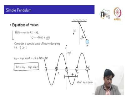
So, let us consider one basic example before moving to the definitions of stability. So, this is a simple pendulum what we have been seeing in you your wall clocks particularly. So, here in the first; so, these two equations defines the basic equations of motions of a simple pendulum where the torque are balances out where Q is the damping torque influenced by the external force u of t, ok.
