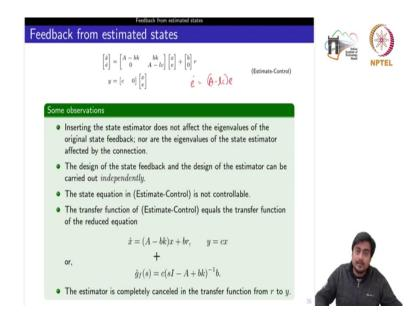
Let us see some couple of more observations. So, this was the estimate control or the closed loop dynamics we have obtained. So, inserting the state estimator does not affect the eigenvalues of the original state feedback nor are the eigenvalue of the state estimator affected by this connection. So, this we had already seen a second. So, as a consequence of this first point the design of the state feedback and the design of the estimator can be carried out now independently.
