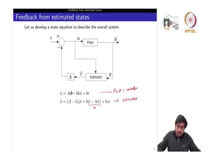
Now, seeing the second equation which is basically the estimator that this is the estimator where we have x hat is equal to A minus lc x hat plus b u. Now here we have also replaced u by r minus k x hat and plus and the last term is l y or we can write y as c x ok. So, this is you can see the plant plus controller and this one is your estimator ok.
