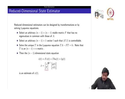
So, here we will see one design procedure which is based on the Lyapunov equation. So, we recall the steps what we had seen in the full order observer there we select an arbitrary stable matrix F of dimension n. But here we select an arbitrary matrix of dimension n minus 1 which is lesser than n.
