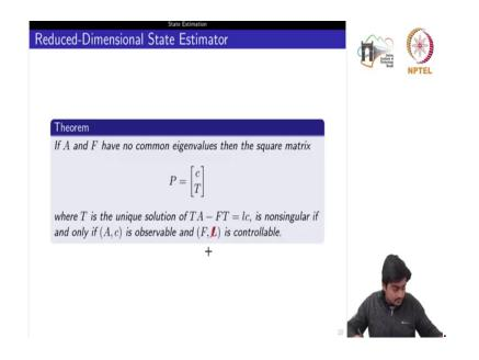
So, this result talks about the non singularity of this P matrix. So, if A and F have no common eigenvalues which we have already ensured in the design step by selecting this F matrix in such a way that the both these matrices do not share the same eigenvalues. Then the square matrix defined by this by combining the c output matrix and the T matrix. Where T is the uniques or where the t is basically obtained by solving this Lyapunov equation ok.
