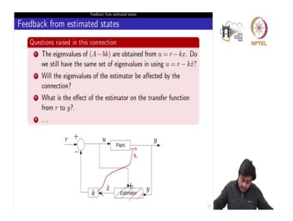
So, after seeing this connection there are some questions which arises naturally. So, the first one is that the eigen values of this A minus b k which we have obtained this matrix after applying only the state feedback are obtained from this one. So, do we still have the same set of eigenvalues in using u is equal to r minus k x hat right.
