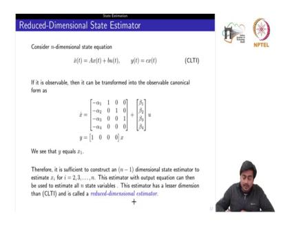
So, today we will introduce the reduced dimensional state estimator, where if x is an n dimension, x is of n dimension then, we need to design the observer whose state is lesser than the n dimension ok. So, if it is possible, then we call those observer as the reduced dimension observer or the state estimator. So, the first question arises here that whether such kind of produce design is possible or not.
