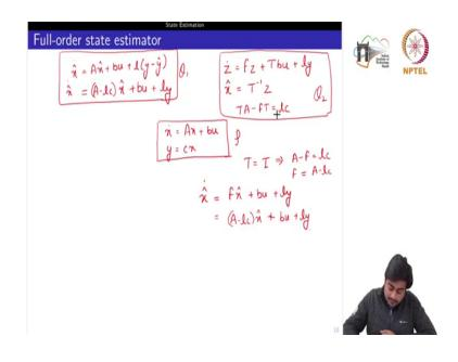
So, in the last lecture, we had seen the two approaches for designing the observer. So, the first observer we had seen is given by x hat dot is equal to A x hat, then we added one term which defines y minus y hat right. And, we also parameterise this in the form of the into this form x hat plus b u plus l y ok.
