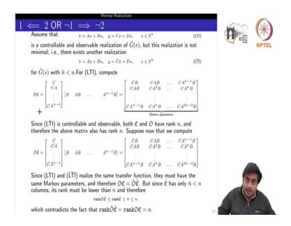
We can also prove this by contradiction meaning to say that assume that ABCD pair is both controllable and observable realization of G hat ok, but this realization is not minimal. That is to say that there exists another realization which is given by this pair A bar B bar C bar D bar in which the dimension of the state x bar is n bar now which is less than n because if this realization is not minimal.
