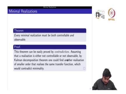
So, this is one of the key result that every minimal realization must be both controllable and observable right. We can see the proof of this theorem by contradiction.
