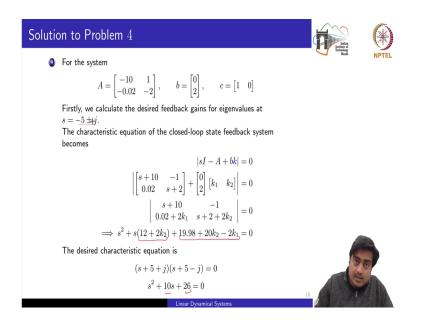
So, for the given information A, b, c we can calculate this eigenvalues, we can calculate the desired feedback gains for the eigenvalues this one. And there are number of methods we had discussed because. Again this is a input controller design. So, you can use either of the designed method, either the eigenvalues assignment approach or the Liapno design base approach, ok.
