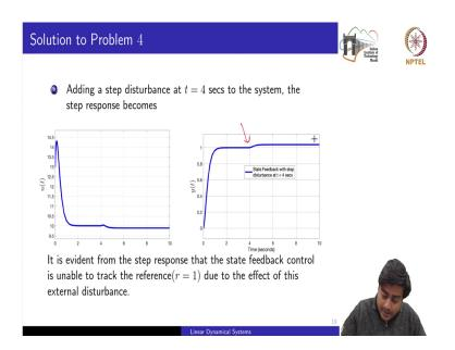
So, this we you can do in simulations also that we have added a step disturbance at t is equal to 4 seconds to the system and the step response or the output of the system is now given by this. So, at the time when the disturbance was inserted into the closed loop system the output was not able to track the reference signal, ok, due to this external disturbance. So, disturbance has some predominant effect on to the closed loop system.
