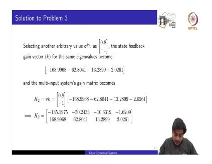
Now, the second matrix second state feedback gain matrix we can compute by selecting another arbitrary vector v, column vector v which is we have selected here as 0.8 and minus 1. Then following the same procedure first of all computing the state feedback gain vector k for us reduced single input system and then computing K 2 as the multiplication of the column vector v, what we have selected here is and the row vector K, what we have compared here.
