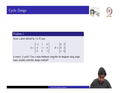
So, in the problem 1 given a plant defined by the pair A, B, where A, B matrices are given by this. So, the first question we need to address to find out whether the matrix A is cyclic or not, and the second part of the question is can a state feedback controller be designed using single input variable control design method, ok.
