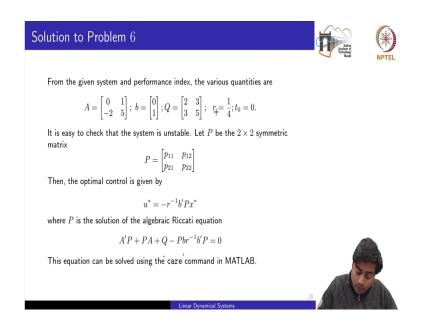
So, let us see if we write our problem into the standard form as we had seen into the lecture slides. So, the matrix A, vector b, this Q would be a state weighting matrix and r since we are using we are having a single input system, so this is a scalar and t naught is equal to 0. So, you can quickly verify that this system is at unstable system by computing the eigenvalues of the matrix A.
