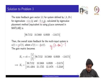
But we want to synthesize this k and we can do this by computing the original control input signal u as v times u dash where u dash is now minus k times of x, ok. So, now, if we compute this K 1 which would be the multiplication of this v vector or v column vector and this k row vector, so we can compute this K 1 matrix, ok.
