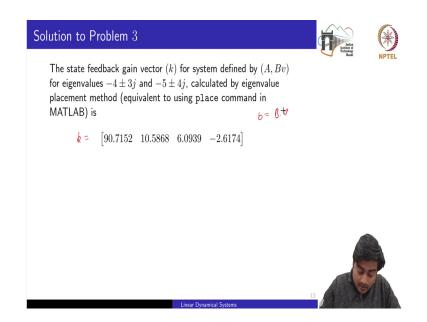
The state feedback gain vector k because we want to synthesize this is a vector k, so that the eigenvalues could be placed at these locations and we can do this by using the eigenvalue assignment method, we had discuss in the lecture or you can use the place command in MATLAB as an alternative. So, this k vector we have computed.
