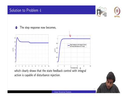
So, now if we pay attention to the closed loop signals of the system on which the disturbances being acted. So, you see when the disturbance is been added at t is equal to 4 the output almost tracks the reference signal now, ok. Because of this new structure we are able to reject the effect of the disturbances on the output signal path. And this happens we know already implicitly because of this integral action which is able to diminish the error between the reference and the output, ok.
