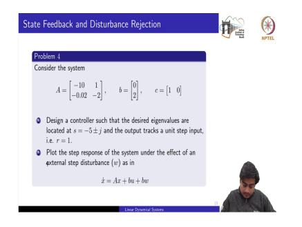
So, in this problem we would see the two points. First of all we will design the state feedback gain which ensure the stability, second we design the feed forward gain such that the another objective which is the tracking objective can also be fulfill, this is part A. And in part B we would see that if there are some external step disturbances happens to be on this system then how the response of the closed loop system would behave, ok.
