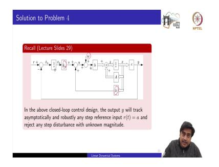
So, we recall the lecture slides where that is 29 on which we have discussed another closed loop architect, another closed loop architecture which ensure that the this external disturbance or the effect of this external disturbance on to y would be nullified, so that two design parameters are k and k a.
