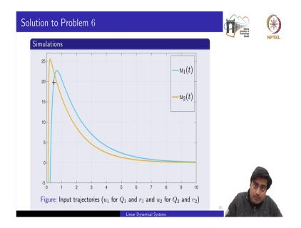
So, by putting this Q 1, Q 2, r 1, r 2 we simulated the scenario and this blue signal is the u 1 and this orange signal is u 2. So, as we have predicted that u 2 would be more regressive because the state trajectories need to reach to 0 as fast as possible, ok.
