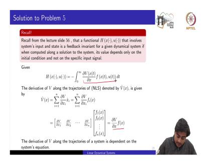
So, recall from the lecture slide number 56, we have defined a functional H is a feedback invariant whenever if when computed along a solution to a system to the system its value depends only on the initial condition and not on the specific input signal. So, this is how we defined any function which involve system input and state as a feedback invariant, ok.
