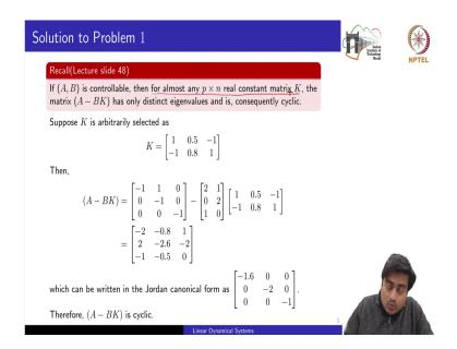
So, it calling again this results it says that for almost any real constant matrix K of appropriate dimension could ensure the of cyclicity of the matrix A minus B times K. So, here we select K is any arbitrary matrix is this one and then computing A minus B times K which happens to be this matrix and we can write this into the Jordan canonical form in this. So, we see that all the eigenvalues are place at the diagonal and therefore, this matrix is a cyclic matrix, ok.
