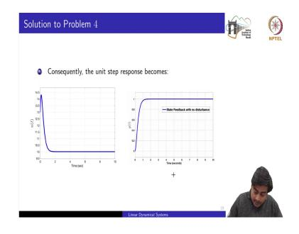
This we can see in simulations also that once I put the controller as u is equal to p r minus k x, the output of the closed loop system tracks the reference r is equal to 1 and this is the control signal, ok. Now, the second part of this problem deals that if there is some disturbances acting
