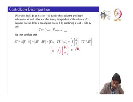
If the system is not controllable, then let us say we define A matrix U. If the system is not controllable it means that the rank is not equal to n, but it is less than n ok. So, we define another matrix U which is an n times n minus n bar matrix whose columns are linearly independent of each other and also linearly independent of the columns of V. So, this U matrix has these two properties that all the columns are linearly independent to each other and also to the matrix V.
