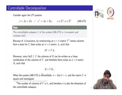
Now, because of the invariance of the or a invariance of the subspace we can construct an n cross n bar matrix V where the n bar is nothing, but the number of columns of V matrix whose columns forms a basis for this controllable subspace um. This is the in fact the one the first property of any linear subspace being A invariant or any matrix invariant here it is A. So, there exists an n bar cross n bar matrix A, c such that this equation has been is satisfy ok. AV is equal to V into A c.
