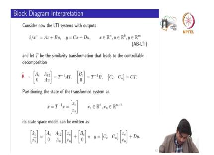
After seeing this controllable and uncontrollable decomposition of the pair AB we can go back to the same representation what we have discussed previously. So, let us see here we have this the LTI system continuous in this part here T is the similarity transformation matrix which decomposed the pair AB into this one and this is nothing, but your A bar pair A bar B bar and C bar and partitioning the state of the transform system as x is x c and x u.
