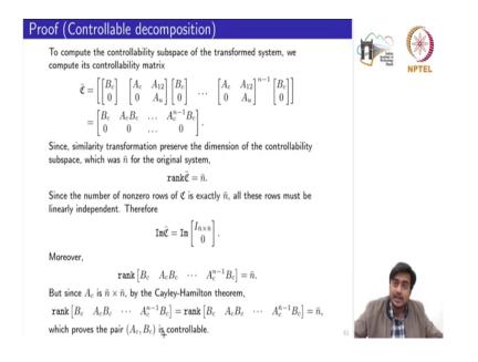
So, to compute the controllability subspace of the transform system, we compute its controllability matrix which is the c bar. Now here I have written all the by opening all these A bar B bar matrices. So, earlier when we studied this controllable decomposition we had over results in terms of bar matrices over it.
