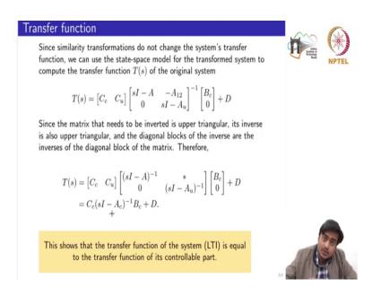
And this of diagonal element we can write we it should be compute, but it is of no use to us because the multiplication of this with this would be 0, ok. So, finally we would have this one C c s I minus A c inverse B c plus D right. So, since you can also use this property that under the any similarity transformation, the transformation does not change.
