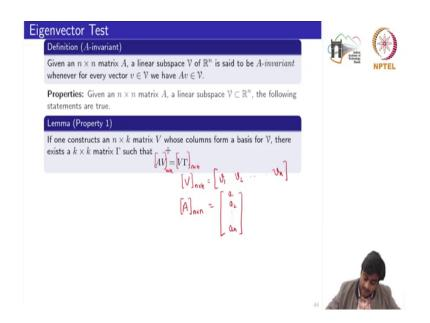
So, there are couple of important properties of this A invariant subspace which we are going to use to state the eigenvector test for the for determining the controllability. So, given a matrix n cross n of dimension n cross n a linear subspace V, the following statements are true. So, I wrote it in terms of the lemma because we are going to see a proof of it as well.
