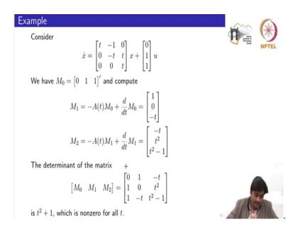
So, this was the weak results. Let us see one quick example so, that you it is pretty much clear of computing the state transition matrices and the additionally defined matrices. So, for example, we are given this A and B matrix where we have specified M naught is equal to basically the B matrix and looking at the dimension of this matrix which is 3; we need to compute 2 matrices M 1 and M 2 by using that formula we have introduced.
