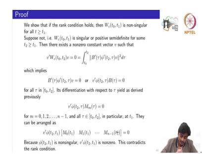
So, we show that if the rank condition holds, that the rank of that matrix then W C t naught comma t 1 is non singular right, because we have we already knew that the controllability of the pair A and B is basically equivalent to saying that the controllability Gramian is non singular ok. So, now, instead of showing that if the rank condition hold then the system is controllable, it is equivalent to saying that if the rank condition holds then the W C matrix is non singular.
