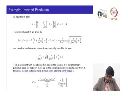
Now, considering at the equilibrium point theta is equal to 0, these are the set of state space matrices we have obtained. Now, the eigenvalues of this matrix A is given by this one and it is quite straightforward to see that these eigenvalues specifically with the positive sign is greater than 0. So, one of the eigenvalues is lying on the writing side meaning to say that the system is unstable and this we can also see while computing the P matrix.
