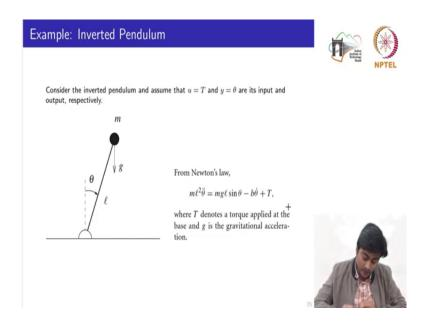
Let us consider one example with which we had started this lecture or this module. So, here we are considering the inverted pendulum. So, there we. So, initially we considered the simple pendulum, but you can also consider it as an inverted pendulum where theta is now the axis the sorry the angle made from the vertical axis, ok.
