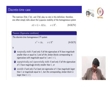
So, therefore, we will mostly speak about the stability of the homogeneous system that is without considering the input. So, for the continuous time system, we studied two conditions, basically 2 tests to determine the stability, one is the eigenvalue test and another is the Lyapunov test. So, the first eigenvalue test for the discrete time system or homogeneous LT I system; so, this x plus denotes the x t plus 1, ok.
