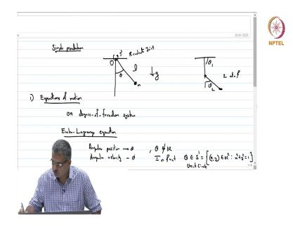
Now, we will assume that there is a torque that can be applied at this joint right of course, we can talk about unforced pendulum or a forced pendulum. So, we will talk about a forced pendulum think of a motor which is which actuates this pendulum right and we will also assume that the pendulum is free to move in the vertical plane it can make complete rotations in this plane right.
