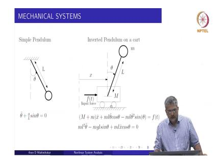
Let us go back go to a simple mechanical system the pendulum the simple pendulum. So, the simple pendulum consists of a massless rod right with the L length L and then there is a the mass is assumed to be a point mass all right with mass m here and the pendulum is it makes an angle theta with d vertical right and the whole thing can move under the influence of gravity.
