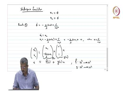
Well now, we have the equations of motion of the simple pendulum right. So, what do we do with this? Well as control systems we will try to put it in state space formulation right. So, the next step is state space formulation. So, state space formulation is not just restricted to linear system one can write the state space even for a non-linear system. So, we have to choose a states for the system.
