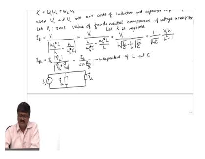
So, there is an I fh which is the rms value of the current of harmonic order h. Now, how to get I fh can I write ifh in terms of I h? Say if you we considered one particular circuit if you just recall, there was a representation of the converter in the form of a current source; I mean we started with this only then the filter is represented by an admittance the network is represented by another admittance.
