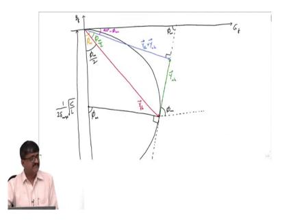
So, we were discussing the Design of single tuned filter. So, let me go to the diagram that we considered in the last class. So, it is the graph of a semicircle where it is shown as a plot in the plane where I have one axis as the real part of the admittance of the filter G f B f. So, we derived some conditions so far. So, we saw that one has to draw a tangent to the semicircle which makes an angle phi m. So, let me draw that tangent.
