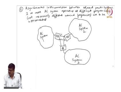
Let us look at some more applications the second application is asynchronous interconnection between adjacent power systems. Now, we say there is an asynchronous interconnection if there are two or more systems operating at different frequencies not necessarily different nominal frequencies, the nominal frequencies can still be same. Now, this comes into picture that is when two or more AC systems operating at different frequencies.
