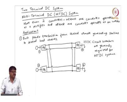
So, these are known as two terminal DC systems. That is a system with 2 converters; one acting as a rectifier another acting as an inverter ok. Now, there are some situations where having more than 2 will be advantageous. So, such systems are known as multi-terminal DC systems, this abbreviated as MTDC.
