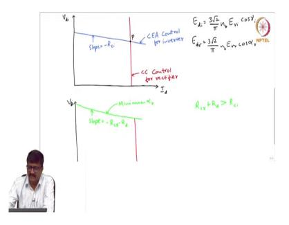
So, it is just a vertical line. So, this is a CC control this is cc control to be more precise I employ control at rectifier for rectifier. Now what do we do at the inverter? What type of control do we employee? See, if I just look at the first control that is the control of alpha r and gamma i. So, gamma i is actually.
