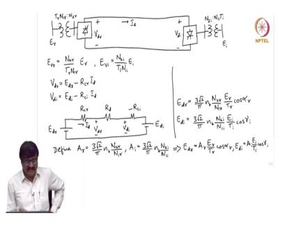
So, this is the schematic diagram of the system. I have the rms value of line to line voltage of the AC bus on the rectifier side as E r. And I have the turns ratio including the off nominal tap T r N 1 r is to N 2 r and the rms value of the line to line voltage of the AC system bus on the inverter side is E i and this is N 2 i is to N 1 i divide N 1 i T i.
