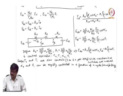
So, changing this T r or T i are slow controls. So, it is essentially a changing the tap position from one step to another step. So, even if you want to change one step of the tap it takes 5 to 6 seconds per step. Because they are mechanical switches since mechanical switches are involved.
