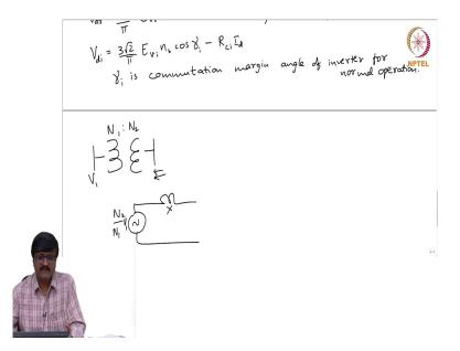
See, if I have, let suppose I have a transformer, ok. Suppose, this is a I mean N 2 by N 1 or whatever ok, N 1 by N 2. So, this is the representation. Suppose, this is V 1 ok, now this representation when you look from this side is a voltage source in series with the reactants like this.
