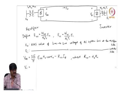
Now, if I want to show a very general arrangement which is common to any of the DC links, I use a different figure. So, I just use this general diagram, again. I again this is another schematic diagram. Suppose I show the rectifier side, so please note now I am slightly changing the meaning of this schematic diagram. This schematic diagram stands for a transformer with box with a rectifier.
