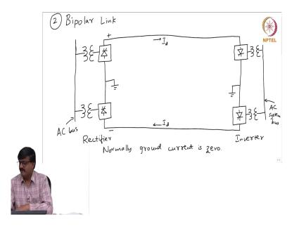
Now, if you look at other go back to any of these links, suppose I go back to say the most common one, bipolar link ok. Now in the circuit, I have an AC bus on the rectifier side, see this is AC this is the AC bus. This is the one of the buses of the AC system. There is another AC bus on the other side. This is the ac system bus. See, one point to notice that this DC link is present in a predominantly AC system, ok.
