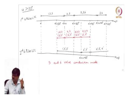
Suppose, u is greater than 30 degrees. So, let me try to again draw a similar diagram. So, I have this one straight line corresponding to omega o t axis for the 6 1 st 6 pulse LCC. Now, if
