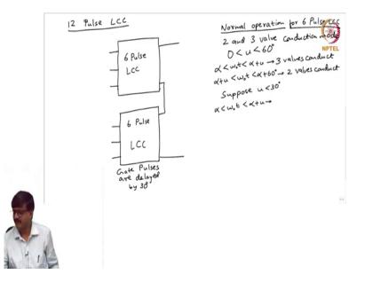
Let us continue our discussion on 12 pulse LCC. Now, we have seen the circuit, I will not try to draw the entire circuit diagram, but what I will do is; I will just show that there are two 6 pulse LCC's in addition to two transformers. For example, I can have one y y transformer and one y delta transformer.
