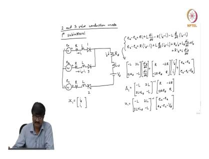
So, if I take 2 and 3 value conduction mode; so, if I take the first sub interval. So, there are 3 valves conducting in the first sub interval. So, I will show only those valves that conduct current. So, the equivalent circuit is like this. This valve 1, valve 3 and valve 2. This is i d, sorry. We have a different circuit now on the DC side, so I have a resistance inductance and a voltage source. So, this is R d, L d, V d. So, how many elements are there in the state vector x 1?
