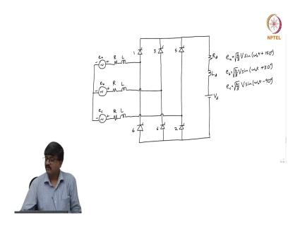
So, the circuit I am considering now is on the AC side I have a 3-phase balanced voltage source. In each phase there is a resistance and an inductance; valves 1, 3, 5, valves 4, 6, 2.
