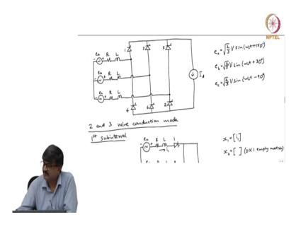
So, we will consider this circuit I have on the AC side a 3 phase balanced voltage source and this is in series with the so in each phase, there is a series resistance and an inductance; R is the
