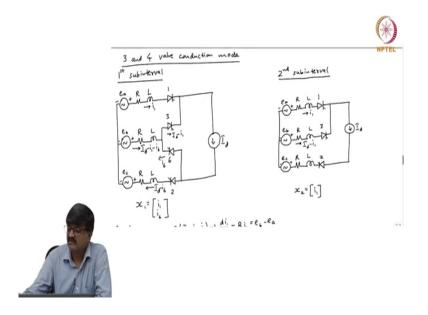
Suppose I consider 3 and 4 valve conduction mode. So, if I take the 1st sub-interval. So, this is similar to the 3 and 4 valve conduction mode of the circuit without resistance. So, the only change now is are the presence of resistance. So, we can see what are the equivalent circuits in the 1st and 2nd sub intervals. So, let us draw the equivalent circuit in the 1st and 2nd sub intervals by just showing those elements which conduct a nonzero current ok. So, in the 1st
