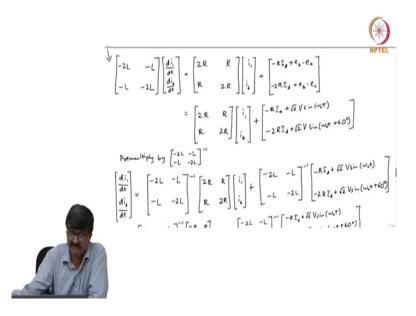
So, I will take a matrix and multiply this by a column vector whose elements are the derivatives first order derivatives of the elements of x 1 that is di 1 by d t and di 6 by dt. So, my intention is to get the equation in the standard form. So, in the standard form I have only the derivative of the state variables on the left hand side ok. So, in both the equations that we have derived so, from these 2 equations I am getting this.
