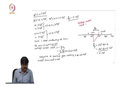
Suppose I take the voltage across valve 1, so, valve 1 stops conducting at alpha plus u. So, that means, up to alpha plus u voltage across valve 1 is 0. So, I will I mean let me also plot the voltage across valve 1. So, let me show some values on the omega o t axis. Suppose this is 90 degrees, this is 120 degrees, this is 150 degrees, say this is 180 degrees, so, alpha plus u is greater than 90 and if I take omega o t greater than alpha plus u and less than alpha plus 120 degrees.
