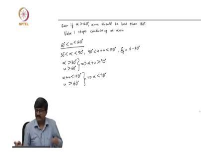
So, even if alpha is greater than 120 degrees alpha plus u should be less than 180 degrees. Now why is it so? Now this is because valve 1 stops conducting at alpha plus u. Now, the condition of minimum value of the commutation margin angle I mean requires that alpha plus u should be less than 180 degrees. So, the reason is same as what was mentioned for normal inverter operation while deriving the expression for the commutation margin angle psi as gamma.
