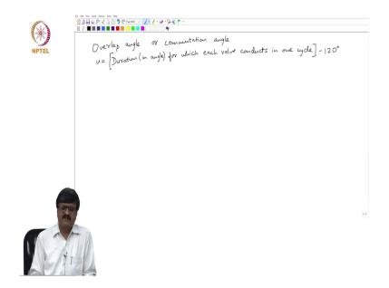
So, we will give a name for that that is known as overlap angle or commutation angle overlap angle or commutation angle. So, we use the letter u for this, the notation is u. So, let us see how to define this. So, the definition is simple.
