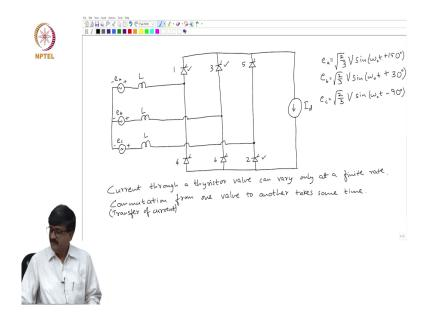
So, let us consider this circuit of course, I have a converter with three legs. The DC side is represented by a constant current source I d. On the ac side I have a three phase voltage source connected in y r star and in each phase on the AC side, there is an inductance the inductances in the three phases are identical. So, L be the inductance.
