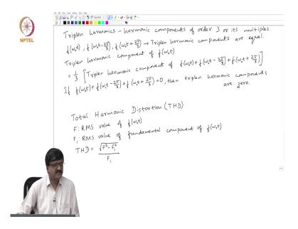
So, there is one set of harmonics which are very important in the AC system that to in the three phase AC system that is the third harmonic sixth harmonic, ninth harmonic, twelfth and so on. So, what I am talking about is the multiple of.
