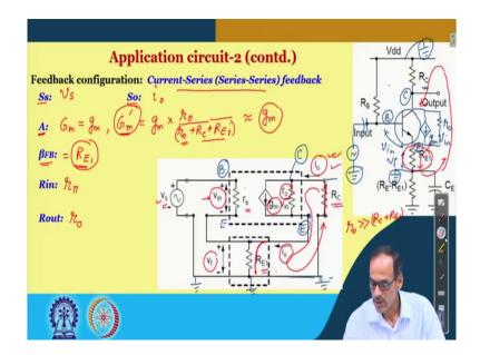
So, if I consider this transistor and if I draw the small signal model, what we have it is Gm into vbe and this vbe it is eventually v in. So, this is v in along with that we do have the resistor r naught and this is the output node, the collector node it is the output node. So, we can see that this node it is collector which is eventually the positive side of the output port.
