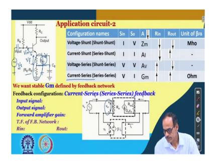
So, what we said is we do have primary input signal here, we call it is v s and then the voltage getting developed here across this R E 1 called v f particularly if we connect the bypass capacitor here instead of this node and of course, this will be AC ground and. So, this is the v f part and then from base to a emitter we do have the input voltage v in.
