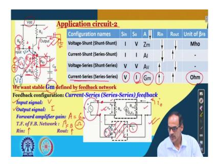
Welcome back after the break into our Analog Electronic Circuits NPTEL course. So, we are talking about Application of Feedback Circuit and in the circuit 1 we have seen voltage shunt feedback and now we do have the second example and we do have the circuit given here.
