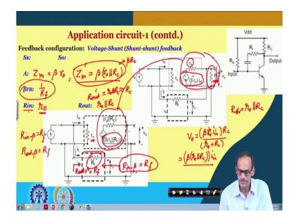
So, we can say that beta FB it is 1 by R f input resistance of the circuit it is r pi and output resistance in this case it is r o which is also getting loaded with R C and typically this R C it is much smaller than r o.
