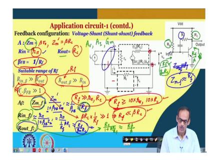
So, in the next slide we are going to do that ah. So . far what I said is Z m it was beta into r o, but more important thing is that Z m f Z m dash rather [vocalised-noise] it is equal to approximately equal to beta into R C and R out dashed it is R C, R in it is r pi, beta FB it is 1 by R f. And then next thing as I said that we need to find what is the suitable range of this R f. And to get that since we are sensing the signal here the voltage.
