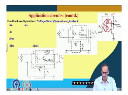
So, here we do have the common emitter amplifier along with its feedback arrangement and we are also adding one capacitor. So, that the DC operating point of the common ammeter amplifier it is not getting disturbed by presence of this R f. So, this R f it is sensing a voltage here and it is providing a current here.
