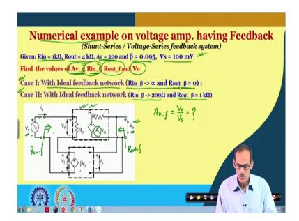
So, welcome back after the break. So here we do have numerical example and what is our objective here? It is that we need to find the voltage gain of the feedback system, input resistance, output resistance of the feedback system and the output voltage for an input voltage or the signal voltage of 100 millivolt.
