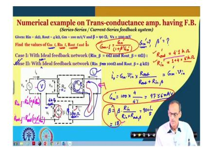
So, I may not be going all the solution for that, but I am going to give you hint for this non-ideal situation, where the input resistance it is 100 ohms and the output resistance of this circuit it is say 4 kilo ohm. So to start with, we need to find what is the corresponding Gm dashed and beta dashed.
