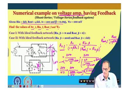
So, if we have say, we need to find what will be the Av f? What we can say that let we postpone the effect of R in beta. So this effect of this R in beta will be postponing. So instead of putting it here, if we connect it here and first we calculate what is the corresponding Av here and then we can consider this part.
