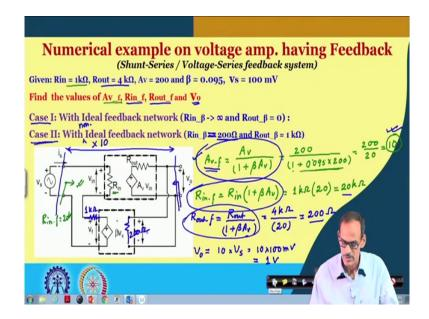
As we know that this Av-f it is the forward amplifier gain Av divided by 1 plus beta into Av. So the Av it is given 200 and on the other hand, feedback factor it is 0.095 and Av it is 200.
