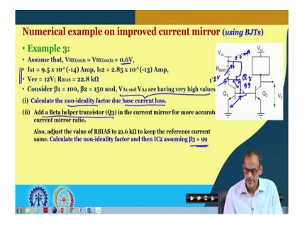
So it is, I should say it is more like a continuation of the previous problem. Namely, we are retaining the parameters here. So, the current flow here it is 0.5 milliampere and we have we have calculated the base current the non-ideality factor due to the base current loss. Now we can improvise the circuit by using beta-helper here.
