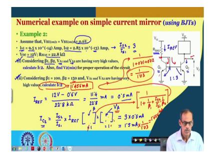
Now, in this example we do have Q 1 and Q 2. Now it is forming the current mirror and in this case, just for a change, instead of giving a reference current, we are giving a resistor here, supply voltage it is given to us 12 volt. This R BIAS register in resistance it is 22.8 kiloohm and then we can assume that V BE on voltage for both the transistors are approximately 0.6 volt. In addition to that, we also have the information about reverse saturation current of the 2 transistors.
