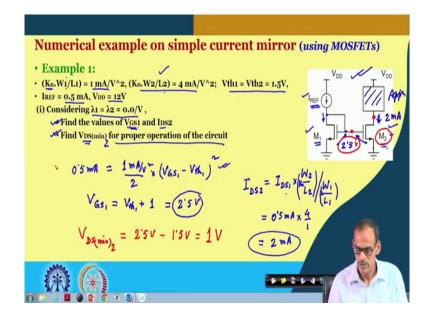
So, here we do have the example circuit where M 1 and M 2 are forming current mirror. We do have a reference current here and then we do have the application circuit here. So in this
