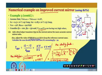
So, here we do have the beta-helper circuit drawn for you. We do have Q 3 here and as I said there this is approximately 0.6 and here also, it is approximately 0.6. So, we do have 1.2 volt. So what we are doing here, to retain this current of 0.5 milliampere in this numerical example, we are readjusting this R BIAS to 21.6 kiloohm And that gives us the I reference current, it is same as 0.5.
