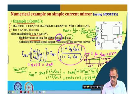
So, in the next slide we do have, so, what we have here it is all the other parameters remaining same. In fact, it is continuation of the same example, but we are considering lambda is equal to 0.01 per volt. And then again, we can try to find what is the corresponding value of this current. And particularly for 2 cases, if V DS2 here that is 2.5 and 5.5.
