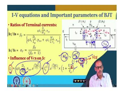
So, let us see how it is getting influenced by the reverse bias voltage at the V BE. So, we do have this V BE; first of all the collector current we are approximating by this component dominating namely the injection current and where we do have the W B. So, this base weight it is basically the residue base weight after deducting and the depletion region both in the emitter junction and the collector junction.
