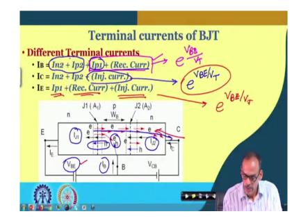
So, as I say that the base terminal current; it is summation of the two current components of this one; namely I n 2 and I p 2. These two indicates the second junction current this is this basically the junction current and also we do have I p I p 1. So, this I p 1; it is again part of this one and that is due to the movement of the holes that is of course, it is not getting change. In addition to that, whatever the d combination it is happening that current is also mentioned here.
