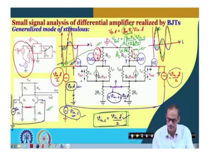
So, in the next slide we do have the generalized mode of stimulous. So, as I said that at the input we like to give both differential and common mode part together. And probably we can make this connection we can make this connection. Now let us see if we apply a differential part here v in d by 2. So, here we do have v in d by 2 and then we do have on the common mode part, let me use blue colour. So, v in c, which is going to going to the to both the inputs.
