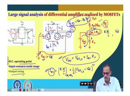
Namely the DC operating point, it is a strong function of the input common mode voltage.
