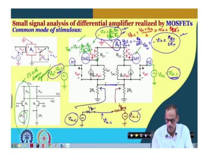
Yeah. So, welcome back after the short break. So, we are talking about the common mode stimulous. And let us see what happens to the circuit, when we stimulate the circuit with identical signal at the 2 inputs. And so, here we do have the small signal equivalent circuit and here, we like to feed the signal small signal. So, v in 1 equals to v in c. So, same thing same signal we are feeding here at the other input.
