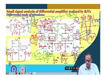
So, we like to put the signal let me use a different color. So, we like to put differential signal here perfectly differential; which means that, here we like to put V in d by 2 and here plus V in d by 2 and both of them are with respect to a DC voltage. And, once we get the small signal equivalent circuit, once we get the small signal equivalent circuit of course, we will be dropping this part and then we will be considering this is AC ground.
