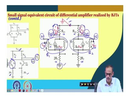
So, just now what we discussed it is shown here. So, what we have it is out of Q 1 we have drawn the small signal equivalent circuit here. So, this is for Q 1. So, likewise we do have the small signal equivalent circuit for Q 2 and then the 2 RT. So, till resistors and then the load resistors are here R C 1 and R C 2.
