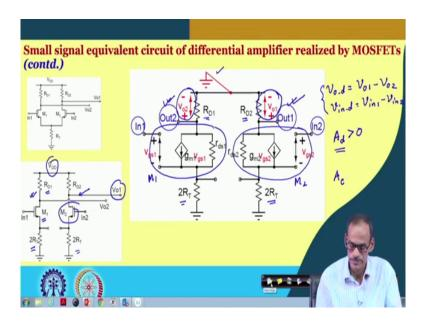
And the two tail resistors split tail resistors are there; and then this node it is AC ground and then this side the drain node of transistor 2, we call it is Out 1 on the other hand drain node of transistor 1 we call it is Out 2. Accordingly, we are declaring this is V o 1 and this is V o 2 and the output we considered particularly the differential output we are defining by considering V o 1 minus V o 2 and V in differential it is V in 1 minus V in 2.
