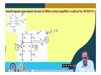
So, in the next slide here we do have the differential amplifier differential amplifier we may consider this one or the customized one here after splitting the tail resistor into identical elements. And, here again we call this is the positive side of the input namely; non-inverting input and this side this node into it is we consider negative side of the input. And, with this we like to declare this is positive side of the output and on the other hand this is negative side of the output.
