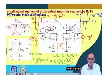
So, this is V o 2 and this V o 2 it is equals to minus V in d by 2 into g m 1 into R C 1 likewise if you see the other side; we do have V o 1 which is in phase with the with the differential input and the signal here it is V o 1 equals to V in d by 2 g m 2 into R C 2. So, the differential output V o d which is defined as V o 1 minus V o 2. So, it becomes V in d by 2 into g m into R C into 2 and here we have assume that g m 1 equals to g m 2 equals to g m and R C 1 equals to R C 2 equals to R C.
