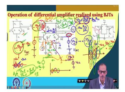
So, now let me let me again summarize what we said here, it is that if we feed a signal at this point called V in 1 on top of a meaningful DC voltage. Let we call V IN C. So, that this meaningful voltage it is ensuring that this transistor it is in active reason of operation. Then the signal we observe at the output terminal, it is V in 1 multiplied by Rc 1 divided by 2 times of R T.
