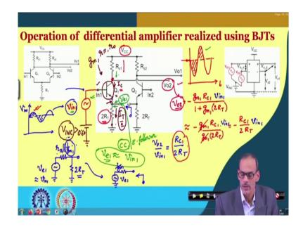
So, let me redraw again clear and redraw the circuit, let you consider we are applying a signal here on a meaningful DC voltage and when we say meaningful DC voltage this DC voltage should be sufficiently high. So, that transistor 1 it is remaining in active region of operation. Now for a meaningful collected current, we need this voltage DC voltage should be at least 0.6 with respect to this ground. So, we are assuming that this V IN C it is higher than Vb on
