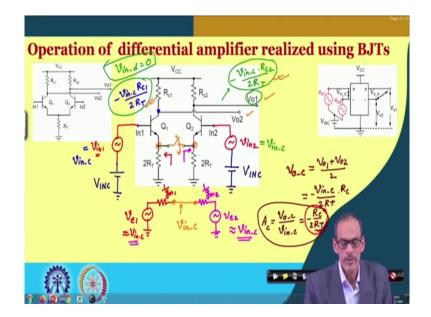
So, let us see for common mode operation. Again coming back to the same circuit, we are applying say V in 1 here and V in 2 here. So, V in one; however, of course, both of them with DC voltage V IN C in capital V IN C and; however, in this case we consider signal here equals to V IN C and also the signal here it is V IN C which means that it is a stimulus in perfectly in common mode operation in other words, we are assuming that a differential input V in d equals to 0.
