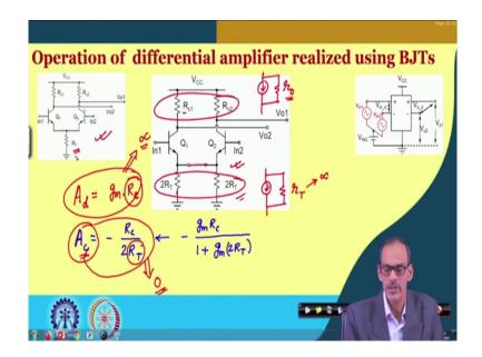
So, the summary of that what do you see, that once you make this connection this circuit and this circuit they are equal and by considering a differential mode of operation, we obtained the expression of Ad which is equal to gm whether it is gm 1 or gm 2 gm multiplied by Rc R c 1 and Rc 2 and the common mode gain on the other hand common mode gain equals to minus R c divided by 2 RT. In fact, to be more precise this expression it is minus gm into Rc divided by 1 plus gm into 2 RT right.
