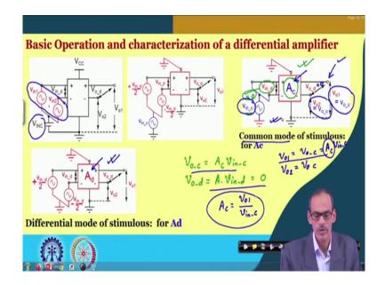
So, in this the second circuit, in the second circuit to find the common mode gain we are making these differential particles to 0. So, naturally, the Voc it is equal to Ac multiplied by V in c whatever the V in c we are applying and Vod on the other hand A d multiplied by V in d. Now V in d equals to 0, so, that gives us Vod equals to 0. And hence the corresponding output V o 1 it is just V o c and V o 2, it is also V o c.
