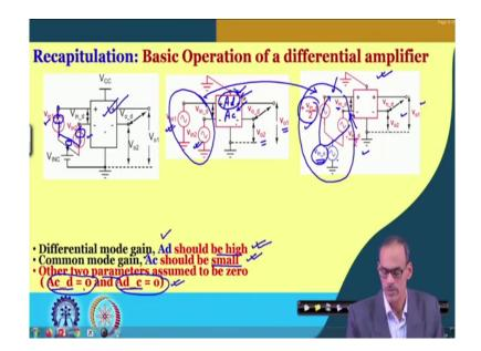
Now once we are in small signal equivalent circuit, then it is basic parameters are differential mode gain and common mode gain as you can see here and we say that ideally we want this differential mode gain it should be as high as possible and this common mode gain on the other hand it should be as small as possible.
