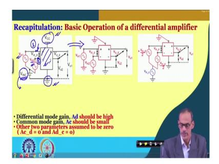
So, to recapitulate whatever we have discussed in our previous lecture we do have say this is a main differential amplifier. Where we have the power supply DC supply and ground and then at the input we do have the differential input port having two terminals 1 and 2 and at this input we are given signal or I should say voltage signal and it is having a DC part meaningful DC part and on top of that we do have two signals. One is V in 1 and V in 2.
