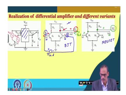
So, how do we realize this differential amplifier. There may be different possible realization of differential amplifier, but here we do have a very basic realization of differential amplifier I should say it is basic, but still it is it is I should say practical circuit.
