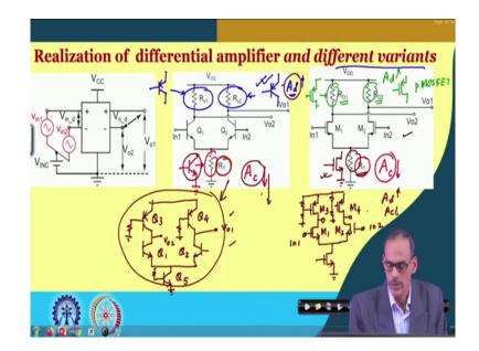
Now, what are the different variants we do have? First of all we have seen that for common emitter amplifier instead of having passive registered we can have active device. So, we can probably replace this passive element by 2 identical PNP transistor. So, here and here. So, as I said that they should be identical. So, and by doing that we can get higher differential gain.
