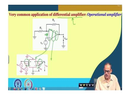
So, to summarize within the within the op amp within the op amp at least it is having a circuit that is the first part the port if you see it is differential. In fact, if you see inside of this, it may be having multiple stages and the first stage it is differential amplifier.
