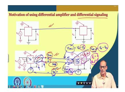
Then how to solve this problem, instead of sending the single signal instead of sending say this kind of single signal, what we can do? We can send the signal which is referred as true signal and its complementary signal.
