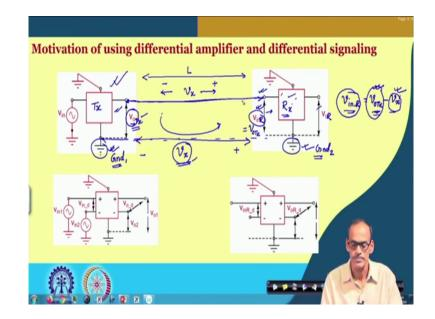
So, in the next slide, we will be talking about the basic need of the differential amplifier. So, suppose we do have single ended amplifier. So, we do have this is one single ended amplifier. And it is producing a signal V out and since it is single ended this V out it is with respect to its common node. And let you call this is the transmitting circuit and then we do have a receiving circuit.
