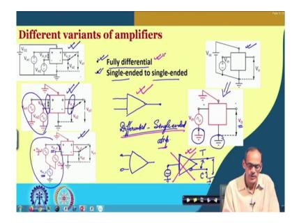
So, here this is the circuit or block diagram of that, here we do have the corresponding linearized model. And here we do have different representation or different way of representing its input signal; namely in terms of the common mode part and the differential part.
