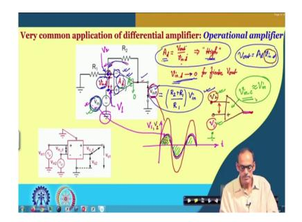
So, let us see why we require differential amplifier for this op amp implementation. Suppose here we do have say op amp having a gain of say A or in fact, strictly speaking it is a differential gain A d. And it is defined by its output vo divided by this differential input v in d.
