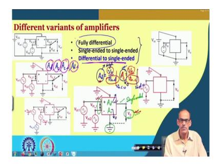
So, in the next slide we are going to give a little hint how this differential to single ended amplifier it is really different. So, if I consider fully differential amplifier, here as I said that there are four basic performance matrices; namely differential mode gain common mode gain and then common mode to differential gain and then differential to common mode gain.
