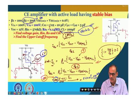
Let us see that. Suppose, instead of taking this value of this resistance half of it. Suppose, this is 1 mega ohm, so that means; instead of taking 570 kilo ohm. In case if it is changing to this value and then what will be the consequence at the output voltage or maybe in case if it is say 1 mega ohm and in addition to that suppose this is getting changed then, what happens?
