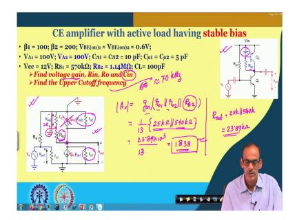
So, here we do have the circuit where we do have this feedback arrangement namely R B got connected to the output node and also we do have this capacitor to fill make the base node not affected by signal coming through this resistor.
