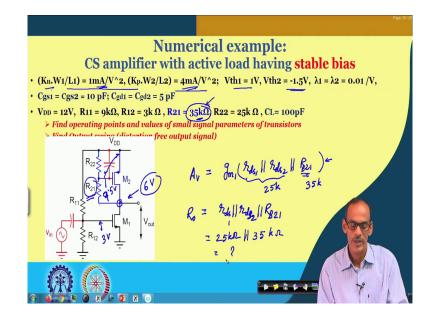
So, here also similar to the BJT circuit, here also the stability issue is there that can be handled by the same approach namely connecting this register instead of connecting to ground we can connect these to output resistance. But then you have to suitably modify this resistance earlier it was 95 k, now we have changed this register to 35 k.
