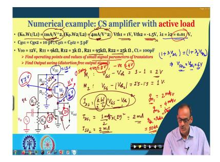
So, we do have here the common source amplifier circuit and we do have the corresponding bias resistors and all. So, if you see this circuit; we do have let me use blue colour, no black colour is fine. So, we do have this register it is 9 k, this resistance it is 3 k. So, that gives us this volt is equal to 3 volt. On the other hand we do have 25 k here and we do have 95 k here.
