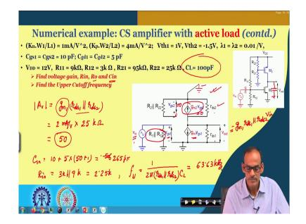
So, we do have the small signal equivalent circuit given here. It is very similar to on the B J T version except of course, we do not have any R pi. So, the calculation here it is I should say simpler and since this node it is connected to A C ground. So, the voltage here it is 0. So, that makes this current equal to 0, leaving behind the circuit is having only r d s 1 and r d s 2 in parallel and then this current incident incidentally V g s 1 equals to this V in.
