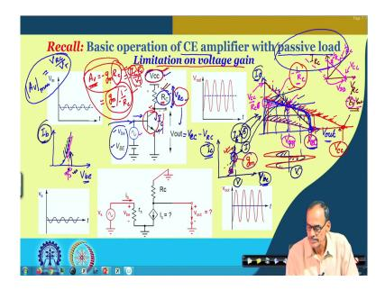
To come to the basic at the base, what we are doing is we are changing the voltage at the base or either you say base voltage or base to emitter voltage. And if you observe the based the current flowing through the base terminal say I b instantaneous current having both DC as well as the small signal part as function of V b e, which is also having a DC part as well as a small signal part. As you know that it is having exponential dependency.
