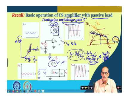
So, as I said that for common source amplifier also we do have the similar kind of problem, to name with that namely the gain voltage gain it will be limited.
