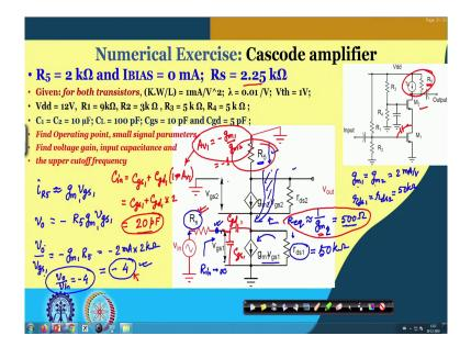
Welcome back after the short break. So, we are talking about the Cascode Amplifier using BJT sorry MOSFET. BJT part we already have completed now come here so, far we are talking about the passive load namely R 5 it was 2 k now we are going to change this load to active kind of load, where our basic motivation is to for higher gain.
