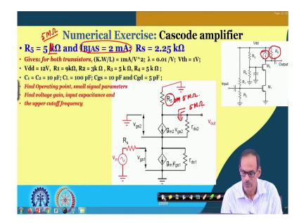
So, we do have; so, we do have the cascode amplifier here with active load namely the I BIAS here it is 2 milli amplifier current and this R 5 it is 5 I should say 5 mega ohm sorry it should not be kilo ohm it will be 5 mega ohm please read as this R 5 as 5 mega ohm.
