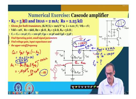
So, to get the input capacitance C in which is C gs plus C gd multiplied by 1 minus whatever the gain we do have from here to here which is let you call this is Av 1 and what is the Av 1? Av 1 equals to minus gm 1 multiplied by rds 1 in parallel with the equivalent resistance coming from this circuit.
