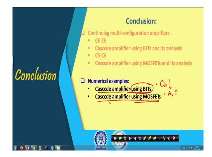
So, today we have in fact, cover only two numerical example, but I guess they are very extensive example to demonstrate the potential of cascode amplifier. First one it is using BJT and we have seen that, it is having both the capabilities. Of course, not simultaneously. So, two capabilities one is it is having the capability to reduce the input capacitance and may be the gain we can maintain same.
