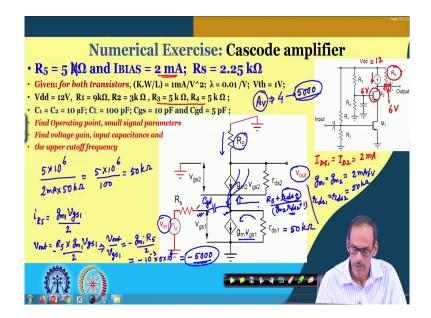
So, the main current it is getting supported by these 2 milli amplifier of I BIAS and then we do have the R equivalent resistance which is matching with this R 5 similar to the bjp BJTs circuit configuration, this 12 volt with this is 5 meg and the equivalent small signal resistance 5 meg, it is giving us a DC voltage here it is half of that. So, that is also 6 volt.
