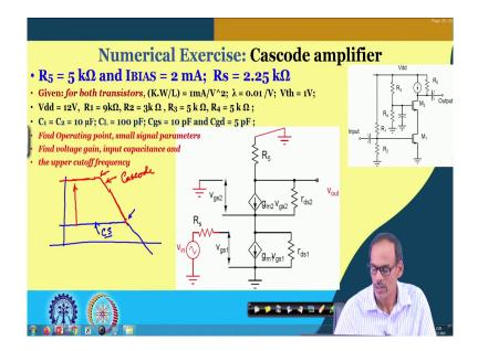
Here the common source amplifier may be having very low gain, but then it may be having very high bandwidth mainly because the output resistance and the CL it is defining that. But then by the virtual of the cascode structure we can increase the gain by a big factor, but then the corresponding bandwidth it is getting affected. So, the gain bandwidth product for both the cascode and the simple common source both may be having the same gain bandwidth product.
