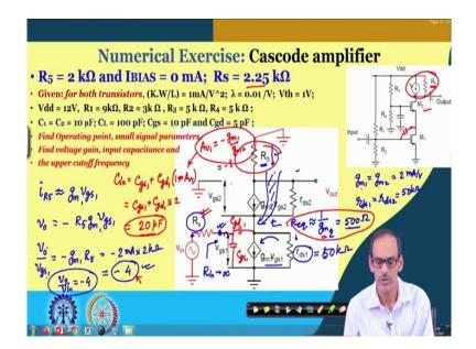
So, let us see in the next slide about the equivalent circuit here and from our previous analysis we see that gm 1 equals to gm 2 equals to 2 milliampere per volt and r d s 1 notation here we are using rds, rds 1 equals to rds 2 is equal to 50 k and the of course, we do not have the r pi here.
