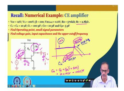
Welcome back after the short break. Before I going to the next topic I must see here that this calculation of the C in I did a small mistake hear, it should be 135 because C in equals to C pi plus C mu into 1 plus 204 and so, here we do have 5 and also here we do have 10. So, I miss this 10 part. So, 10 plus 1025. So, that gives us 1035 pico Farad capacitance.
