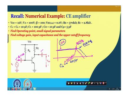
So, the gain if I say that, for CE amplifier gain may be, overall gain it is 102; if I start from here till this point considering the source resistance of 1.3 k. And then the upper cutoff frequency you have obtained here, it was 237 kilo Hertz. On the other hand if I consider cascode amplifier, the gain it was very close slightly higher slightly higher. Note that this is in ratio we need to convert into d v and then the bandwidth here it was remaining; the bandwidth
