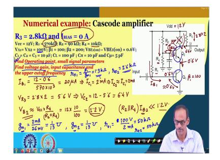
So, to start with let we yeah, let me use different color here. So, to start with we do have here it is supply voltage is 12 volt and then we do have R 1 which is 570 kilo ohm and then we do
