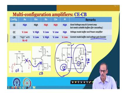
So, we do have the CE stage here and then we do have the CB stage as the name suggests that the output of the CE stage we like to feed it here and if we are feeding the voltage here and there may be a different possibilities, we may remove the capacitors or at least we can say that we can keep only one capacitor. So, if I am putting one capacitor here, then the corresponding configuration becomes like this.
