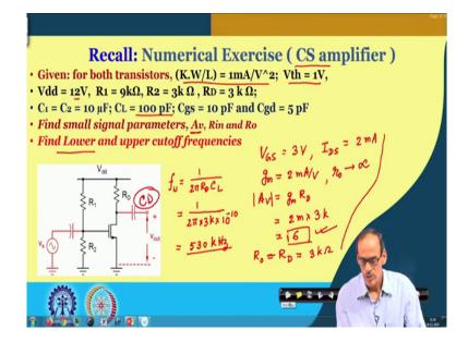
So, in the next slide we will be talking about see common source amplifier again this numerical exercise we have seen before. So, this is prime and the main common source amplifier and sorry and then we have the information given here about the device namely K into W by L which is 1 milli ampere per volt square, threshold voltage it is 1 volt, supply voltage it is 12 volt and so and so.
