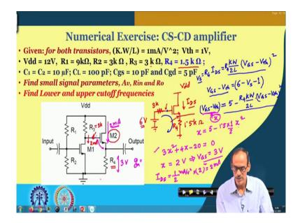
So, we do have in the next slide we do have that example here. So, all the information's are we are keeping it same we do have additional C common drain stage coming out of the transistor M2 and the its bias circuit R 4 and R 4 it is given here it is 1.5 kilo ohm
