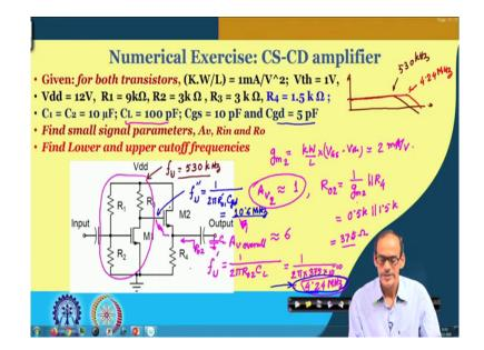
So, the gm of this transistor it is let me create some space here. So, gm of transistor 2 it is we do have KW by L into V GS minus V th. So, here also we got g m 2 equals to 2 milli ampere per volt and then the output resistance and of course, since we do not have the equivalent whatever R pi we are having in BJT.
