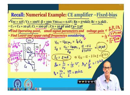
So, let us go to the numerical example. So, this slide is a recapitulation of one of our previous numerical examples where we have discussed about CE amplifier having fixed bias arrangement and different different parameters are given here including the supply voltage of 12 volt, then device parameters including beta of the transistor, early voltage, then V BE on and then also we do have the bias circuits resistances are given here R B then collector resistor and so and so.
