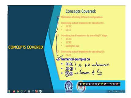
So, here again the same summary here the concepts we already have covered particularly the theoretical aspects of mixing different configurations are covered. And, we are going to discussed about numerical examples of particularly for CE followed by CC common collector stage to enhance the bandwidth of the amplifier and. So, similarly for MOS counterpart common source followed by common drain, it gives the enhancement of the bandwidth.
