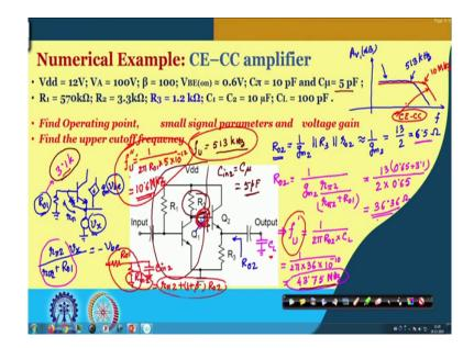
So, let we consider the output resistance here. So, if I call this is R O2 ideally, if the this node is AC ground then R O2 should be equal to 1 by g m 2 in parallel with R 3 in parallel with r o2. So, that we may approximate by 1 by g m 2 and that is 13 by 2 that is point 6.5 ohm, but then this is not possible. We cannot do the AC ground here. So, we have to consider the corresponding resistance here.
