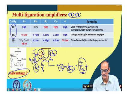
So, the same configuration namely CC followed by CC. So, we do have the CC followed by CC and so, we do have the Q 1 here, we do have the Q 2 here and this is connected to V dd. The output impedance so, we know that this will be in the order of 1 by g m and in this case g m of the second transistor. So, now, the g m of course, it is function of the current ah. So, we do have g m is equal to I C divided by V T or rather one by g m it is V T divided by I C of the second transistor.
