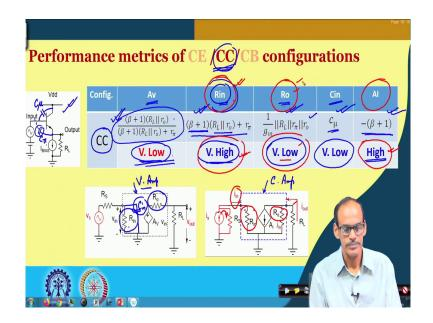
So, let we go to the next slide where we are summarizing common collector configuration. So, we do have common collector configuration it is given here and for this circuit also we do have detailed derivation of the voltage gain, input impedance, then output impedance, then input capacitance and of course, the current gain. And, whenever you are talking about different parameters we do have the corresponding model here voltage amplifier. So, this is for your reference and then current amplifier.
