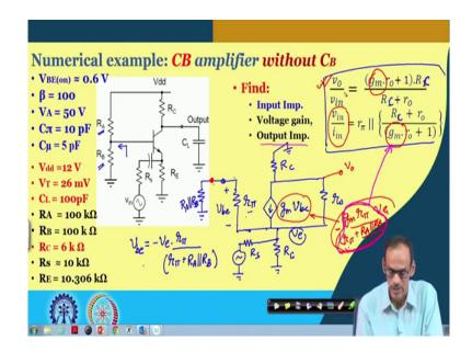
So, this is R C connected to AC ground. So, this is R C this is also R C this is also R C and here we do have g m into v be voltage dependent current source and then of course, you do have the r o and then we do have the RE connected to ground.
