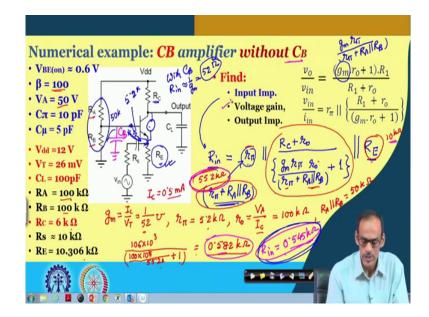
So, what we said is this g m will be replacing by g m r pi divided by r pi plus R A in parallel with R B. So, from that we can say that input resistance R in if I ignore RE and if I consider v in by i in. So, directly we can use this equation and we can see that this is r pi in parallel with R 1 is basically R C. So, R C plus r o divided by g m into r pi divided by r pi plus R A in parallel with R B right multiplied by r o plus 1.
