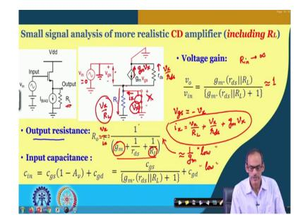
So, if I want to know what will be the output resistance, let me use red color, yeah. So, we have to make it this is ground and then we need to stimulate this circuit by say v x and then current flowing through this is i x and the moment we are applying say v x here the current
