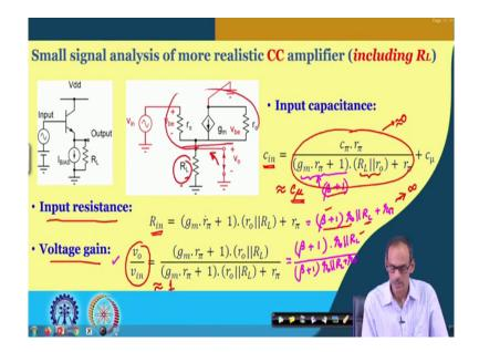
In fact, you can further simplify this one wherever we do have the g m into r pi you may replace this by beta of the transistor. So, here also we can write this is beta plus 1 into r naught in parallel with R L plus r pi. So, likewise here also you can write this part you can write beta plus 1 into this one. So, similarly for the voltage gain here you can write in terms of beta instead of g m and r pi, so we can say that this is beta plus 1 into r o in parallel with R L plus r pi.
