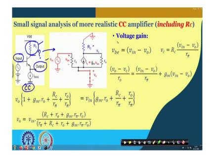
So, what we have it is, yeah. So, here we do have the circuit the corresponding circuit, we do have the common collector circuit having this R c connected to V dd. Note that, please do not get confused that output still remains, the output terminal is basically the emitter of the transistor even though we do have a meaning maybe some signal coming to the collector terminal, but we may not be really concerned about this signal unless otherwise it is stated.
