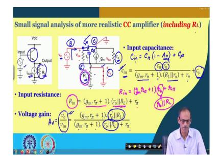
So, to start with let we let you consider the common collector amplifier and also in the common collector amplifier we are including this R L. So, this R L may be coming from the bias circuit, representing the finite conductance of the bias circuit or maybe and or maybe additional load resistance we are connecting at the output node with respect to ground.
