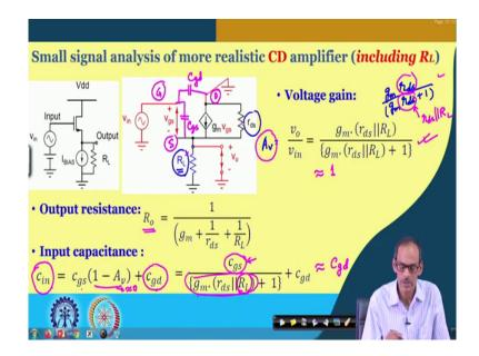
So, the common drain stage considering R L and its voltage gain, voltage gain it is given here. So, again you may recall the previous analysis where we have not considered R L, for that the voltage gain it was g m into r ds divided by g m into r ds plus 1.
