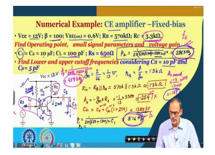
So, in the next slide we do have CE amplifier having fixed bias arrangement and different components of, so different components of these bias as well as the other value the capacitors and all it is given here. So, R B, R B it is 570 kilo ohm, supply voltage it is 12 volt and then V BE on it is approximately 0.6. So, that gives the base current equals to 20 microampere.
