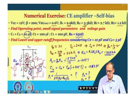
So, I will be giving little hint to solve this problem. First of all here again we shall try to find the operating point of the transistor. So, if you consider R 1 of 9.9 k and R 2 it is 3.3 k. Again, the voltage coming here it is 3 volt. So, we do have the value of this resistance it is 9.9 k and we do have 3.3 k, so that gives us 3 volt here. And with this 3 volt if you consider that we do have the base to emitter voltage drop of 0.6, in fact, that gives us this voltage equals to 2.4 volt.
