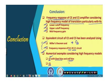
So, in summary what we have so far we have covered it is. So, in this module what we have covered here it is basically we have considered high frequency model of transistor and particularly in presence of source resistance R s, what is its impact on the frequency response of common emitter and common source amplifiers. And what you have seen primarily, it is the change of the lower cutoff frequency and upper cutoff frequency and also the mid frequency gain.
