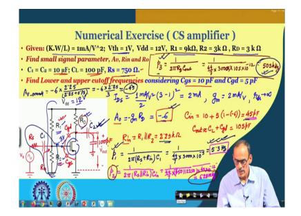
So, again this circuit is very similar, but we need to be careful here that g m of this transistor MOS transistor, since it is much lower than g m of b j t, so we are expecting the gain here it will be much lower and then we can see what is its consequence in the frequency response.
