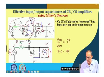
What we have what I said is that from here to here the gain it is defined by A naught, in addition to that we do have this resistance coming in series with or getting loaded by net output capacitance called C out. On the other hand, from this point to this point if we see the
