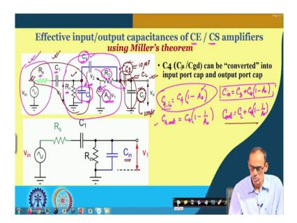
Yeah. So, welcome after the break. So, we are talking about the, in fact, what we got it is the generalized model of CE and CS amplifier here. What it is having here it is the input signal source, having the source resistance of R s, and then signal coupling capacitor C 1, and then if I consider this is the main amplifier where we do have the input resistance represented by this R 1.
