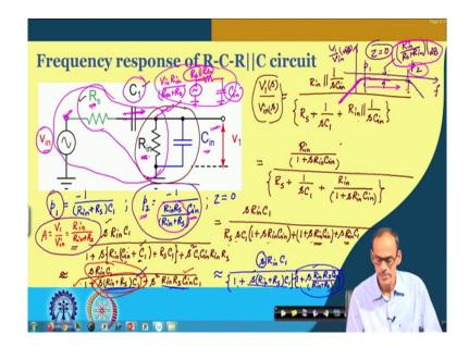
So, we do have this circuit, we do have R, and then C, and then R and the C coming in parallel. Now, if you see here to get the frequency response of this circuit namely in Laplace domain V 1 s divided by V in s we can get the transfer function by considering this impedance which is R in, in parallel with 1 by s C in and then R s in series with 1 by s C 1 plus R in parallel with 1 by s C in.
