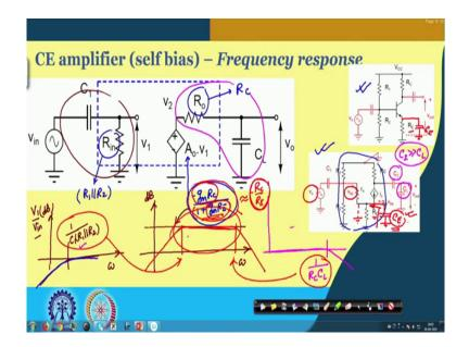
So, then if you see what will be the overall frequency response; now, as we said that this is the this is the small signal circuit where the core portion we have discussed just now and what we have obtained that the gain here, the amplifier gain here it is a g m into R-C divided by 1 plus g m into R E with a minus sign. So, this is the gain A naught.
