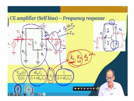
So, you may recall that in this self-biased circuit we do have the emitter resistor and so and also the at the base we do have R 1 and R 2 from this V cc to generate one DC voltage here. And then of course, the signal it was coming here through this signal coupling capacitor C 1, at the output we do have the C 2.
