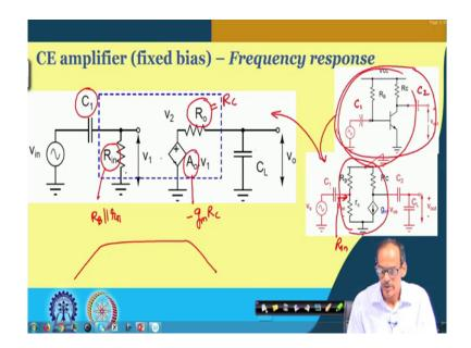
Now, again just for a slight recapitulation; in case, if you recall the fixed bias circuit where this is the circuit diagram given here, which is having coupling capacitor here C 1 and C 2 signal coupling capacitor and then we have drawn the small signal equivalent circuit of the amplifier which is basically the core part.
