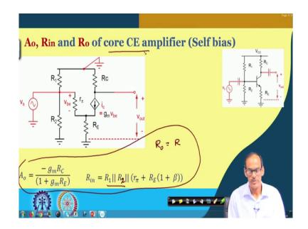
So, what we said here it is this should be R 2 and in addition to that R o equals to R-C. So, this informations these three expressions basically the information about the core CE amplifier, we are going to use to get the frequency response of this entire circuit.
