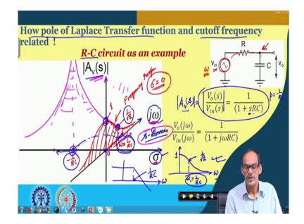
So, this is what the we are about to discuss that the transfer function pole of transfer function in Laplace domain and the cutoff frequency they are related. And, let us consider this simple R-C circuit which is having one pole and the location of the pole, it is if you see here the location of this pole it is p equals to minus 1 by RC which means that s is equal to minus 1 by RC the transfer function the magnitude here it will be going to be infinite.
