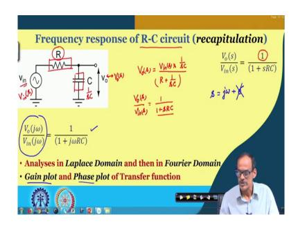
So, similar to the C-R circuit again here what you are doing is that we are taking the circuit into Laplace domain, namely the impedance of both the elements we are going in Laplace domain for C it is 1 by s into C and this is directly same as this R. And then input it is V in Laplace domain s and then the corresponding output also we are considering in Laplace domain which is V o s.
