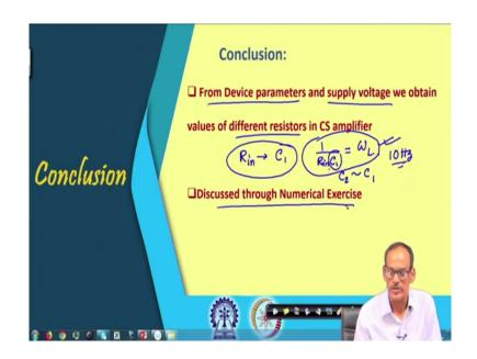
So, the what are the things we have covered here it is basically from the device parameter and the supply voltage information. And, if we start with a meaningful current then we can find the value of different registers. Once we find the resistances particularly input resistance from that you can find what will be the corresponding C 1, because if I combine these two namely
