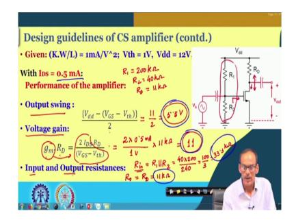
So, the performance which whatever the design just now we obtained namely the R 1 equals to 200 K and then R 2 equals to 40 K and R D equals to 11 K. What are the performances matrices we are getting? First of all the output swing V dd minus V GS minus V th by 2 which is actually 11 by 2; that means, 5.5 volt. The possible swing here it is actually plus minus 5.5 volt right and the corresponding gain what we can get is gm into R D.
