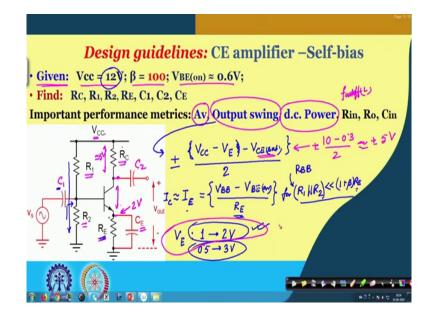
So, here we do have self-bias and here again we are assuming that these informations are given to us namely, the supply voltage is given to us V BE on it is coming from the data set, the beta also may be coming from the datasheet or it may be you can use multi meter or by some other means to find the value of beta.
