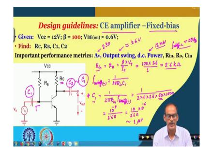
Then, R in approximately equal to r pi which is beta divided by g m which is I C divided by V T. And, if I consider I C is say 1 milliampere as a special case or one case and beta is say 100. So, from that we can say that beta multiplied by 26 millivolt divided by 1 milliampere. So, this gives us 2.6 k all right.
