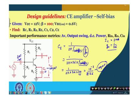
So, let me clear and then write it about the expression of C E need to be followed. So, C E it is 1 by 2 pi then the f lower cutoff frequency, and then of course, the resistance which is 1 by g m of the transistor. So, we have seen that this 1 by g m it is for say 1 milliampere of current
