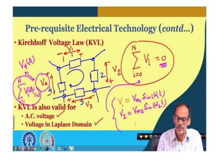
So, this is what we like to say. Similarly for KVL also; so, for KVL also we can deploy the this KVL for AC signal in that case of course, the signal it will be voltage and also the signal may be even in Laplace domain. So, there also we can use KVL. So, quickly just to complete
