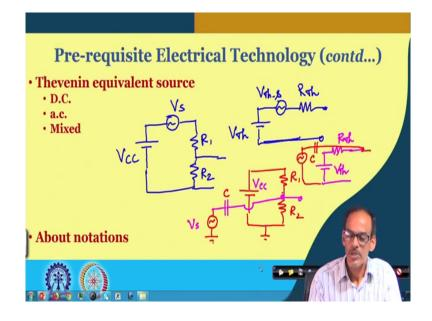
To start with we do have a say DC source and then we do have AC signal and then you do have the potential divider and then you can find what maybe the corresponding Thevenin equivalent voltage source and so and so. Note that this situation it is fairly simple and straightforward. So, whatever Vcc we do have and then signal source you do have a both of them are seeing the same circuit. This analysis it will be simpler you may say that I do have a
