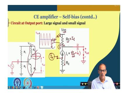
So, let me go to the; so, here again we do have the large signal and a small signal notion. And, here we do have the; here we do have the actual circuit and at this point we do have the voltage shown here and we are going to talk about at this circuit along with this DC decoupling capacitor.
