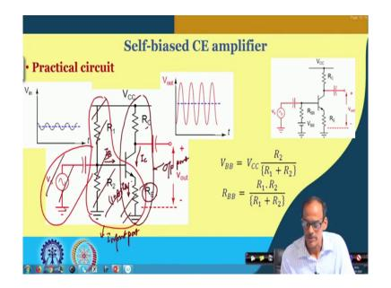
So, if I consider input port is this one DC wise, in addition to that we do have the signal. And, the output port we do have on the other hand consist of on the collector register, transistor and also this emitter register. So, you need to see that this emitter register it is part of the input, input port as well as the output port as well as the output port.
