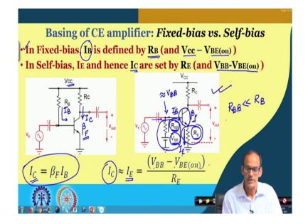
So, as we have discussed that this is the; this is the fixed bias kind of circuit and here what we have done it is the base current, base terminal current particularly the DC current I B it is decided by the V CC and then V BE on and this R B. So, in fixed bias circuit the base current it is well defined by the base register called R B and then supply voltage minus base to emitter diode on voltage.
