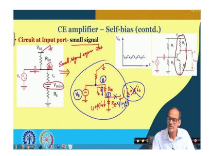
So, I do have a different slide for that. In fact, the same circuit we are drawing here, but what we are talking about; we are going to talk about the small signal analysis. So, once we have this entire circuit and we like to see what will be the corresponding small signal equivalent circuit; equivalent circuit.
