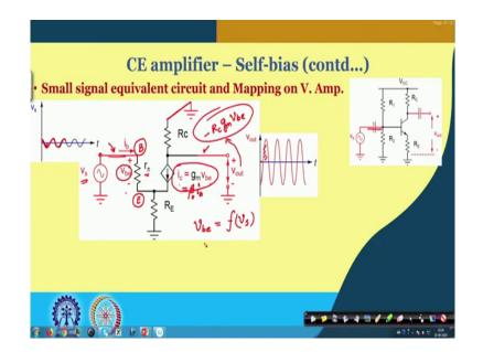
So, let us see what you are going to get here yes. So, we do have this small signal equivalent circuit shown here, where now if you see at the collector side we are making AC ground first thing. The capacitor here we are shorting; so, that is what we are doing and then the collector current it is having only the small signal collector current, small i c which is g m times V be.
