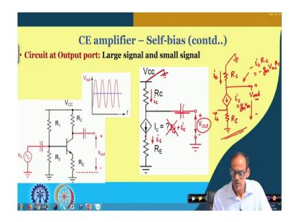
And similar to the input port here again for small signal what are the things we will be doing, it is the this terminal will be will be considering AC ground. So, this is AC ground and here
