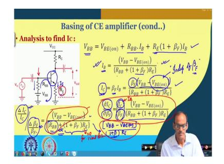
So, in the next slide we are going to analyze this circuit in detail. So, what we have here it is we do have the same circuit we have discussed we do have V BB. Now, if I consider say this loop, this loop then we can say V BB equals to V BE on plus drop across this resistance which is R BB multiplied by I B plus the drop across this emitter register R E. And the drop here it is of course, the resistance multiplied by the emitter current I E.
